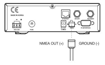
Figure 18: NMEA 0183 GPS Connection
