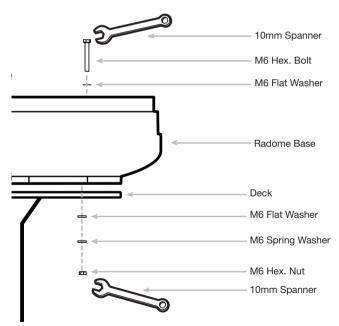
Figure 12: Mounting the Antenna
