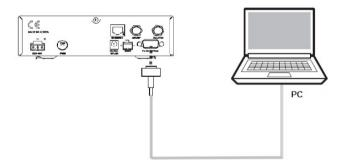
Figure 22: Serial Connection
