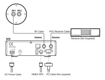
Figure 15: Single Receiver Configuration
