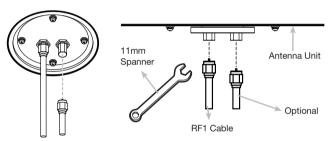
Figure 11: Connectors on Bottom of Antenna
