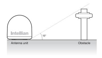
Figure 07: Elevation Limit of Obstacles
