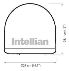
Figure 08: Radome Dimension of i2
