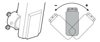
Figure 21: Manual Angle Adjustment LNB Skew
