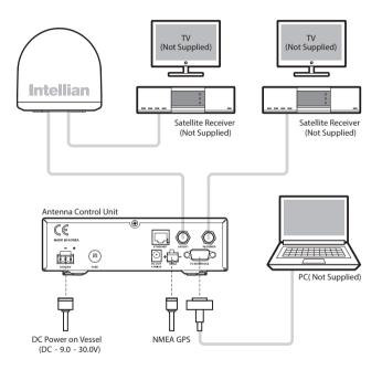
Figure 01 : Basic Configuration with 2 Receivers
