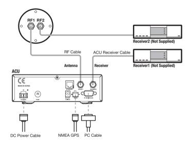
Figure 16: Dual-Receivers Configuration
