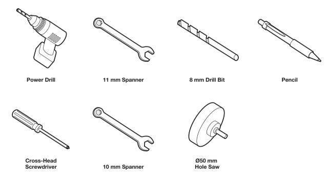
Figure 06: Required Tools for Installation
