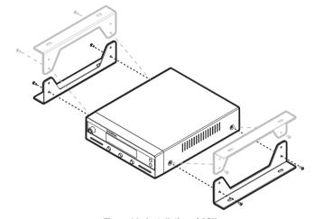
Figure 14 : Installation of ACU
