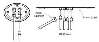
Figure 11: Connectors on Bottom of Antenna
