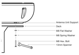
Figure 12: Mounting the Antenna
