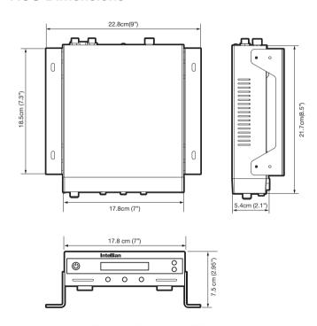
Figure 13: Dimension of ACU for i6W
