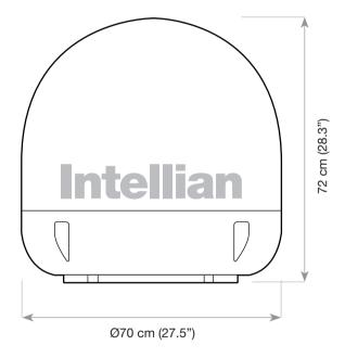
Figure 8: Radome Dimension of i6W
