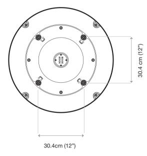
Figure 9: Mounting Hole Position of i6W
