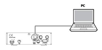
Figure 23 : ACU to PC TCP/IP Connection
