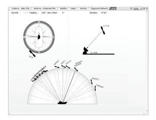
**Note:** Based on the satellite EIRP footprint and the size of the antenna, you may not be able to track all the satellites visible in 180° arc.
