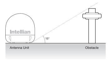
Figure 7: Elevation Limit of Obstacles
