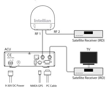
Figure 1: Basic System Configuration
